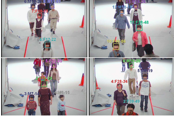
Figure 7. Sample screen shots of the real-time human profile recognition system.
