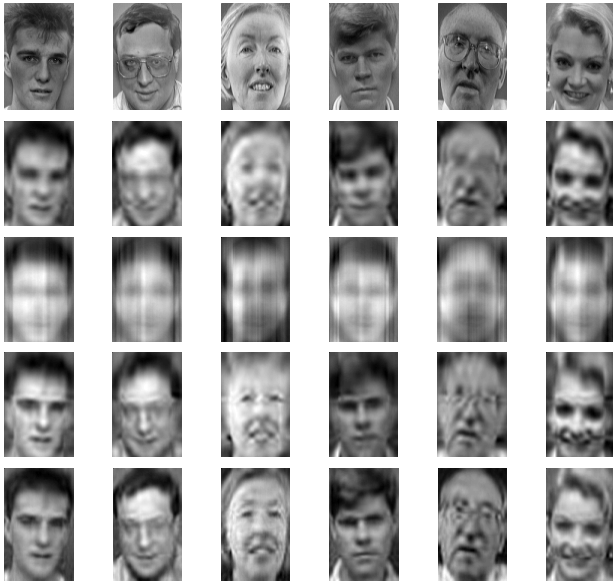
Figure 1: Reconstructions of some ORL face images. row1: original images; row2: using general PSOPCA; row3: using (right) one-mode PSOPCA; row4: using PSOPCA with FA noise model. row5: Mixture of PSOPCA with 5 components. The projection dimensions are r = c = 15 .
